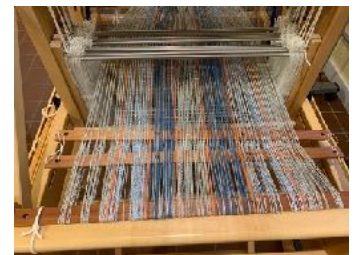
7. Warp Transferred to Back Beam and Lease Sticks transferred behind reed
