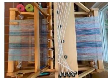
9. Completed beaming viewed from above (Cont'd page 5)
