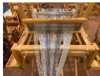
8. Warping in Progress (Yank and crank method)
