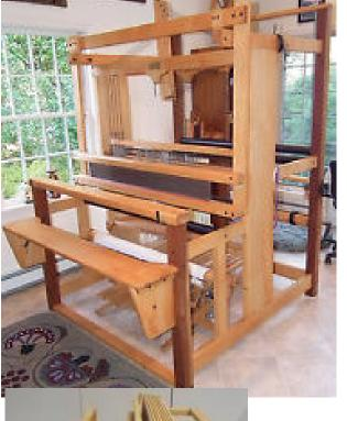
60" Collingwood - Harrisville Rug loom, 8 shafts with shaft switching device, two back beams 800 heddles, 10 treadles, with a footprint of 76" wide, 72" deep and 82" high. Has a 24" warp extender for longer warps. Shipping weight including crate: 650 lbs, Full width Shaft switching device 25 lbs Asking price: \$10,600 & comes with a full width Shaft switching device
